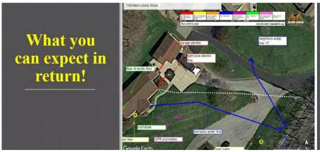
The dotted line is their bore path – would have dug into one their water line without having a
